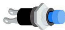
Push-to-break switch The switch is off while the button is pushed, but returns to its 'on' position when button is released.
