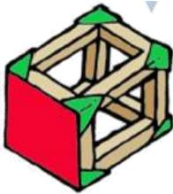
Attach thick corrugated card to 5 of the faces, leaving one side open to view the CAM mechanism.
